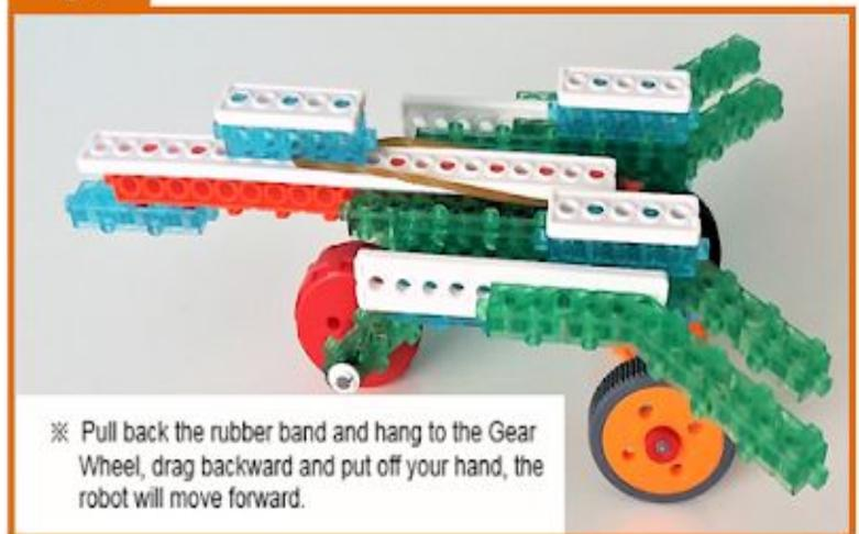
※ Pull back the rubber band and hang to the Gear Wheel, drag backward and put off your hand, the robot will move forward.
